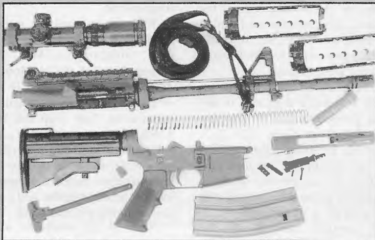
M16A3 M4 Carbine, fieldstripped.
